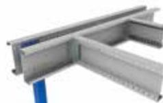
A rigid L-connector makes the joint between the main beam and the secondary beam. The loads from the secondary beam are transferred to the main beam without any deformation of the connector.
