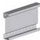
The secondary beam is a sigma profile, designed to ensure that it is hardly sensitive to torsion under load. A full range of sigma profiles of high quality micro-alloy steel are available. The type of wooden decking or grating, its size and the load capacity determine the span between and the type of secondary beams.
