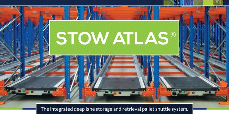
The Stow Atlas® pallet shuttle system is a deep lane storage and retrieval system. It utilises a carrier to move pallets within a specifically designed racking structure, thus optimizing the storage capacity.
